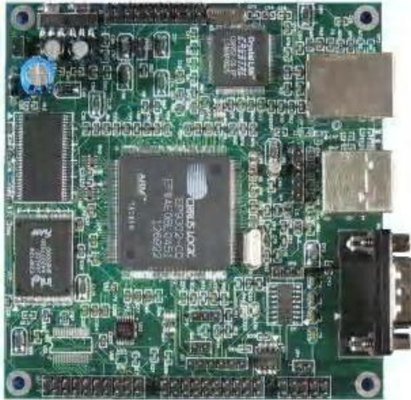
Figure 1. GESBC-9302 Single Board Computer
